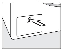
Press the drain pump access panel.
